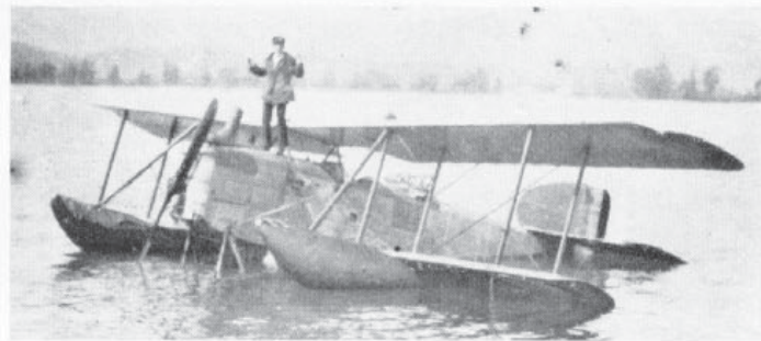
Breguet 14B2 fitted with flotation gear. The aircraft has horn-balanced ailerons, wire trailing edges, the late 14B2 lower wing and underwing skids.
