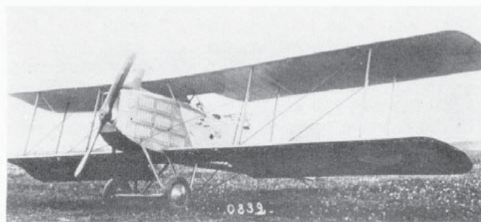
Two views of an early Breguet 14B2, No. 670. The three-quarter front view shows the greater length of the lower wing; both illustrations show the lower-wing flaps clearly. This aircraft had not been fitted with Michelin bomb racks and their characteristic forward projection of the lower-wing leading edges when this photograph was made; there were no windows in the fuselage sides at the observer's cockpit, and his gun ring was a T.O.4. No shutters were fitted to the radiator at this stage.
