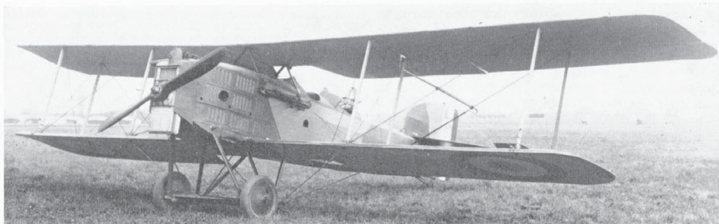
Fiat-powered Breguet 14A2 with enlarged radiator.
